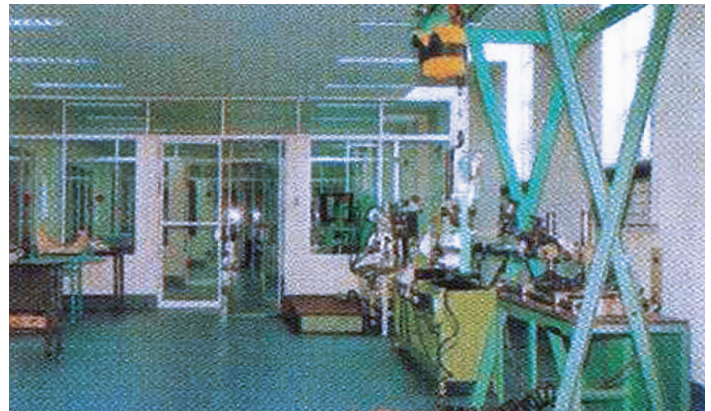
Air-conditioned dust free facility provided for coil making and insulation taping
